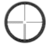
Filar/bifilar reticle pattern
